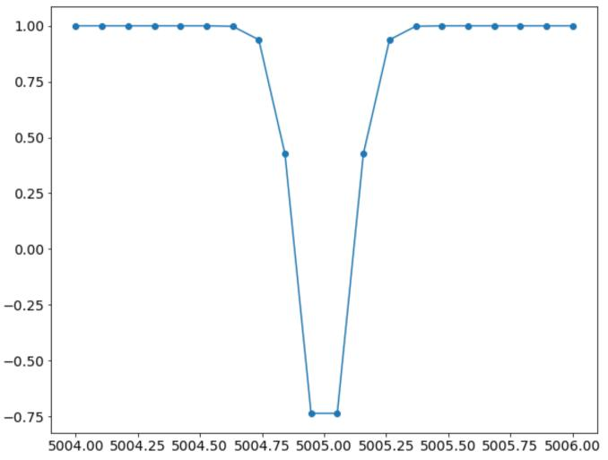
Spectral line with width 0.1 A, spectral resolution 0.1 A
